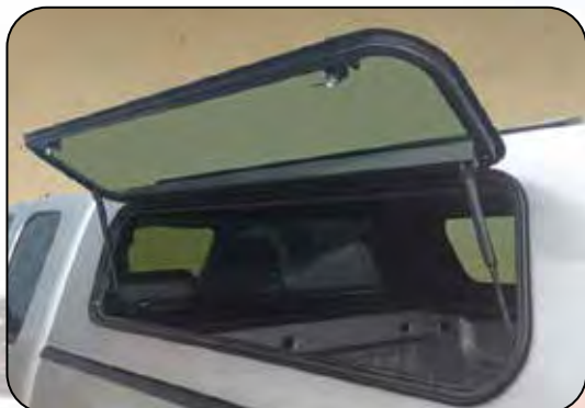
Optional side Windowor provides added access to cap interior
