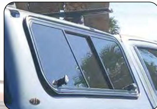
Optional side Windowor with Slider provides ventilation without opening the entire window
