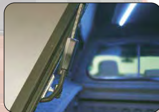
Optional Switch for Auto On/Off Lighting
