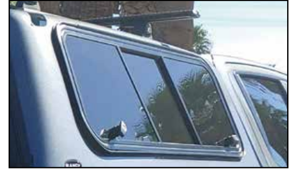
Optional side Windoor with Slider provides ventilation without opening the entire Windoor
